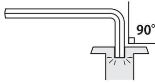
When you use the allen key, make sure it is at 90 degrees and is at the bottom of the hole.
