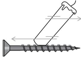
To make assembly easier use candle wax on the screws.
