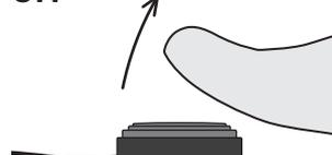
The e-Spinner Super Jumbo will operate only while your foot is on the foot switch. Lift your foot off and the e-Spinner Super Jumbo will stop.
