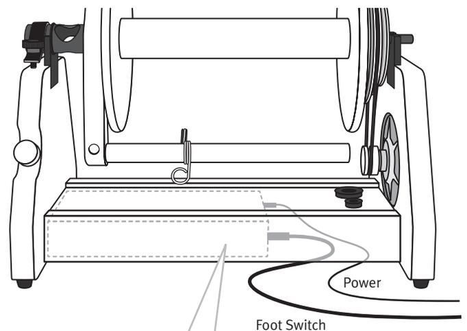
**NOTE:** ensure the e-Spinner Super Jumbo is switched OFF before removing the foot switch plug.
