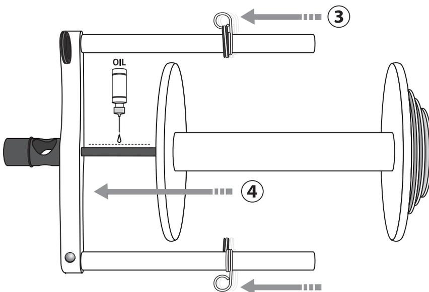
5. Locate the drive band onto the MIDDLE groove in the bobbin whorl. Do not use the large groove as this will stretch the drive band. We have used the Country Spinner2 Bobbin as standard on the e-Spinner Super Jumbo, so they are interchangeable between the two spinning wheels.
