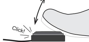
Lightly tap the foot switch to turn the e-Spinner Super Jumbo ON and lightly tap again to turn it OFF.
