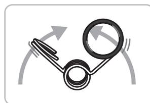
**2.** Cut the nylon brake band into 2 pieces, 35 cm for the brake band and 65 cm (14" and 25 1/2") for the lazy kate. Tie the 35 cm (14") piece to one of the springs attached to a screw eye. Then tie the spring to the brake band allowing approx. 270mm – 280mm (10 1/2 – 11") between the springs. See illustration. Thread the tail of the nylon brake band down the inside of the spring & trim off surplus.
