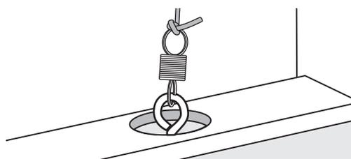
**4.** Thread the screw eye into the pilot hole in the right-hand side.
