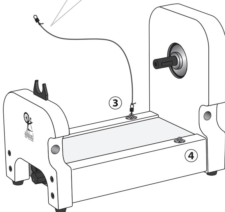
**5.** Apply a drop of oil to the flyer spindle and slide a bobbin on.
