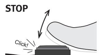
Lightly tap the foot switch to turn the e-Spinner 3 ON and lightly tap again to turn it OFF.
