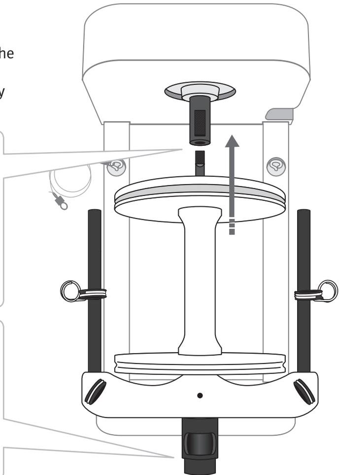
**7.** Tie one end of the black waxed thread to the end of the spring, thread through the screw eye and tension knob and tie a knot.
