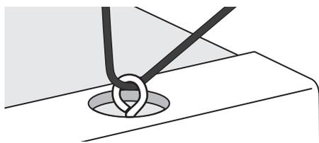
**8.** Place the nylon brake band around the bobbin whorl, place the tension knob in the tapered hole and tighten until the springs just start to extend. This is the normal amount of brake band tension required. Do not extend the springs more than 1 1/2 times their own length.
