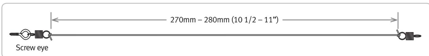
**3.** Thread the screw eye with the tension spring and brake band attached, into the pilot hole in the left-hand side.
