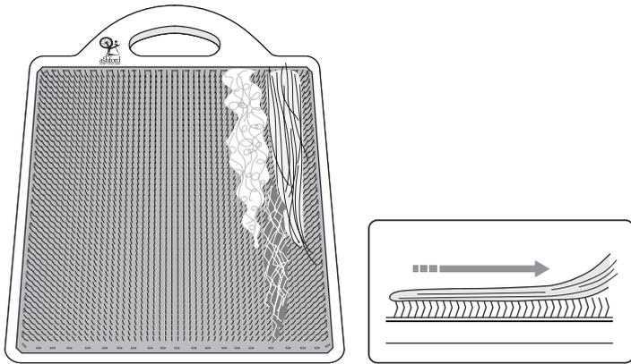
3. Starting at the handle end, apply thin layers of fibre onto the teeth mixing colours and fibres as you go.
