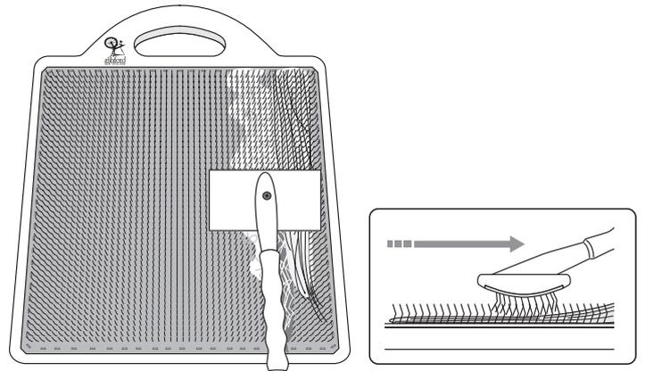
4. Use the blending brush to pack the fibres down into the teeth. Apply more layers of fibre and brush into the teeth until the board is full.
